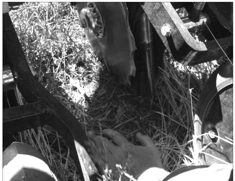
Tim Woods & Graeme Hand inspecting the results of sowing cereal rye into red grass on “Mt Nanima” with a converted Horwood Bagshaw combine, using double disc openers with press wheels on 12” spacings.
