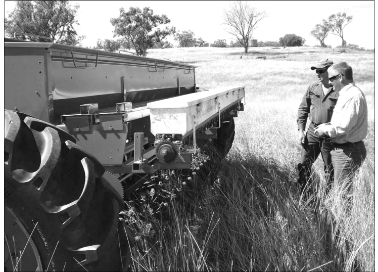
Tim Woods & Graeme Hand inspecting the results of sowing cereal rye into red grass on “Mt Nanima” with a converted Horwood Bagshaw combine, using double disc openers with press wheels on 12” spacings.
