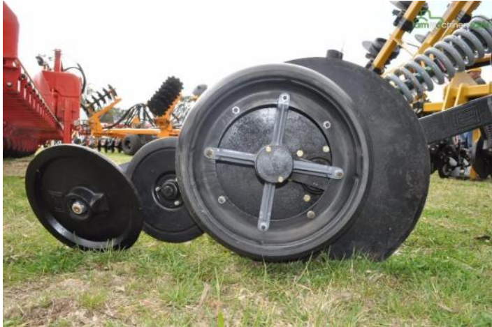
Single disc opener like the type Gabe Brown uses. Photo: Farm Machinery Sales
